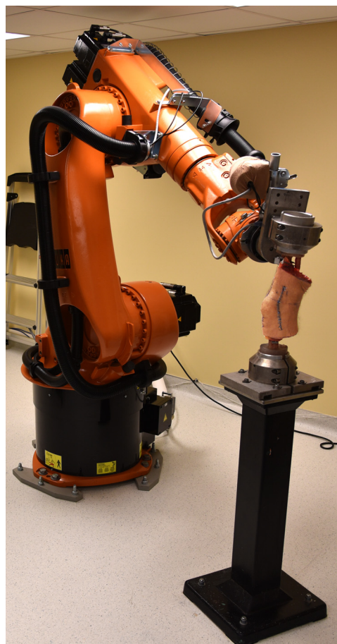
Figure 4 Photograph of a right knee inverted and mounted into the pedestal of a 6° of freedom robotic system for anterolateral ligament reconstruction biomechanical testing. (Color version of figure is available online.)
