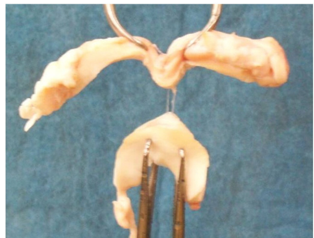
Fig. 3. Horizontal mattress suture repair failure due to suture cutting through the meniscus.
