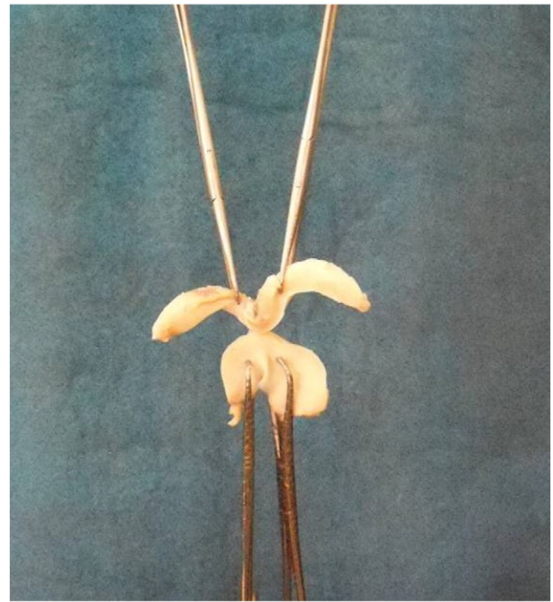
Fig. 2. Biomechanical setup for isolated testing of tensile loading on the meniscal suture repair construct where both portions of the repaired meniscus are held with metal clamps attached to the testing machine.
